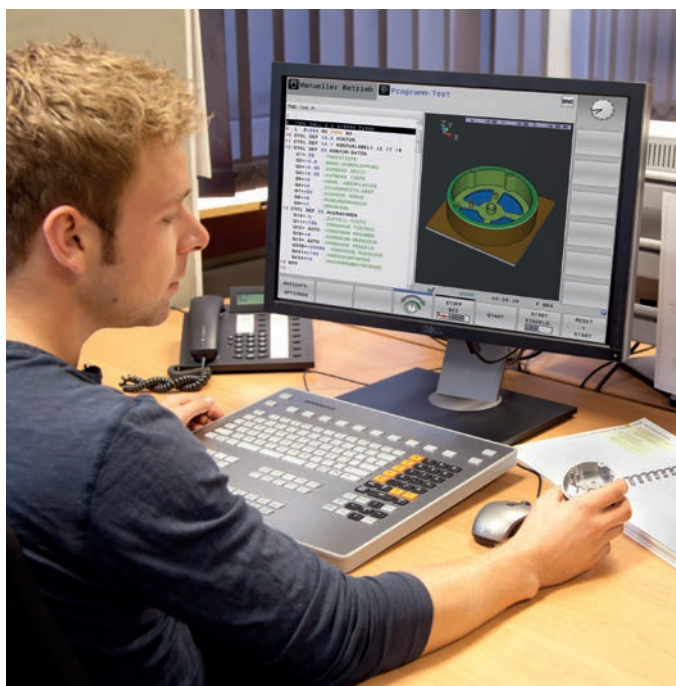
Programming station with TNC operating panel
